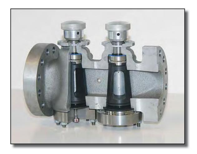
The CCR System avoids overpressure in the cavity between the two plugs, if an emergency situation should occur – if the cavity pressure should increase – due to an explosion, fire ect. The Pressure against the bottom cover will cause the studs to stretch and then open up for relief back into the feed pipeline, and no dangerous gasses/mediums will escape out into the atmosphere. When the pressure falls again the studs retract the bottom cover back to normal position, which closes the bore.
