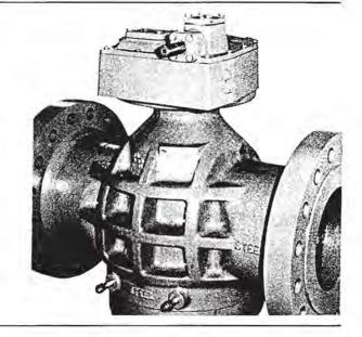
Gear, type D, is enclosed in a water—proof casing, with the handwheel located horizontally on top of the valve.
